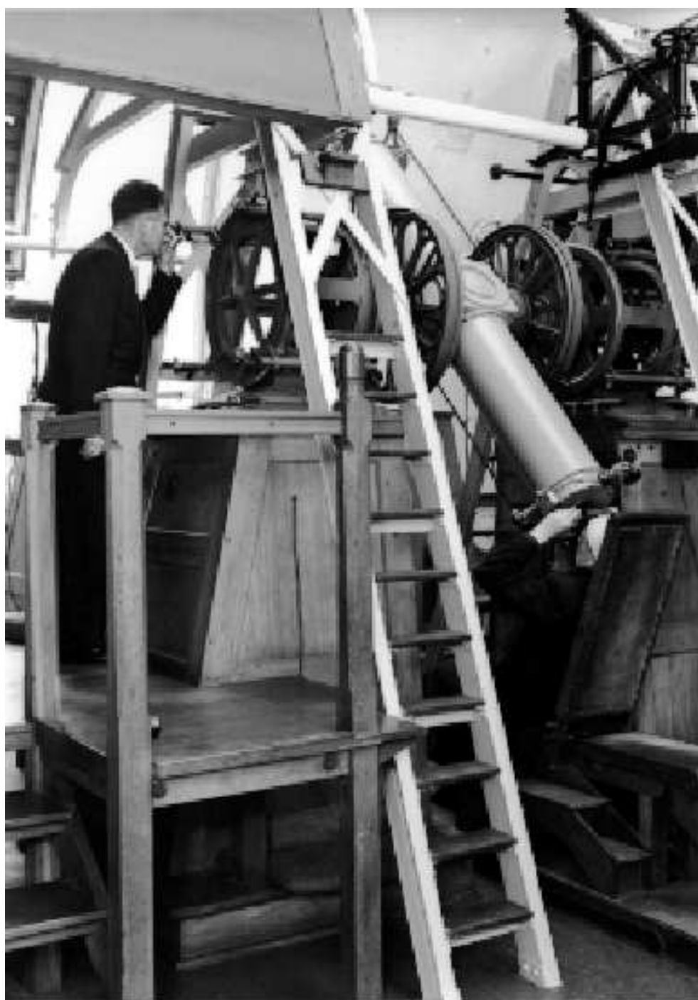
Figure 8.1: Meridian circle (19 cm), A. Repsold & Söhne, Hamburg, 1909 (Perth 1967 bis 1987) Hamburg Observatory
