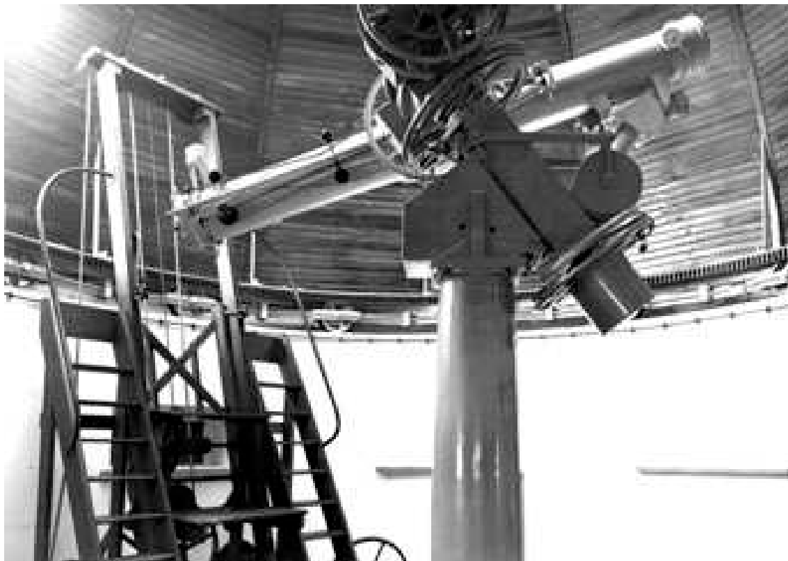
Figure 3.2: Equatorial telescope (26 cm, 3 m), 1867 and observing chair, Repsold, 1909 Optics: G. & S. Merz, Munich Mechanics: A. Repsold & Söhne, Hamburg Hamburg Observatory
